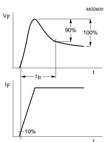
Fig.7 Forward recovery time definition.
