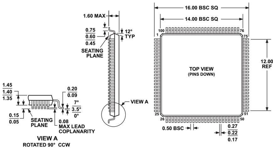
Figure 41. 100-Lead Low Profile Quad Flat Package [LQFP] (ST-100-1)
