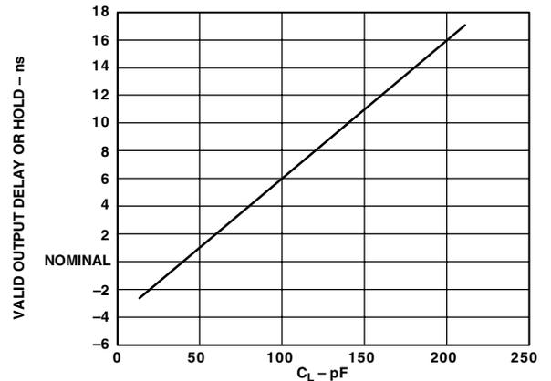
Figure 25. Typical Output Valid Delay or Hold vs. Load Capacitance, C<sub>L</sub> (at Maximum Ambient Operating Temperature)
