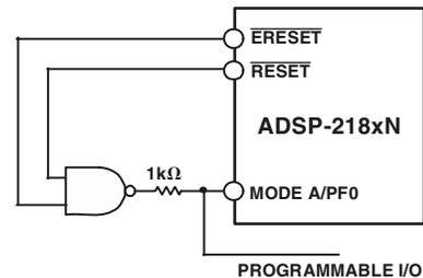
Figure 15. Mode A Pin/EZ-ICE Circuit
