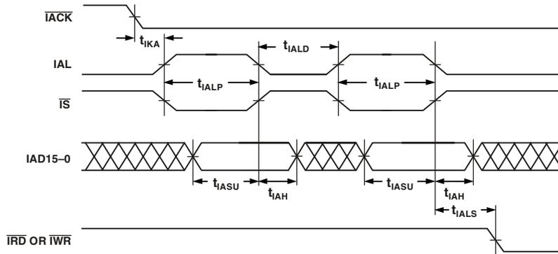
Figure 32. IDMA Address Latch
