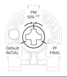
Wiper positioning on initial position is standard. Special delivery positions available on request.
