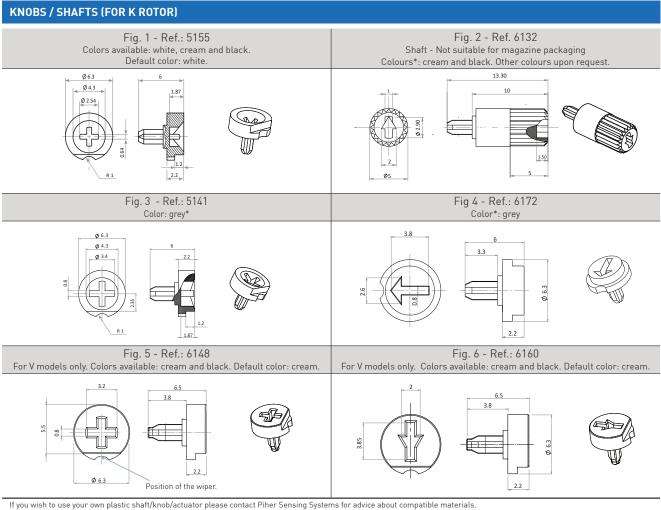
Shaft and knobs (Fig 1 to 4) are delivered unassembled if not specified otherwise in part number code ("W" or "X"). The position of assembled knobs can be indicated in part number code: Initial (default), 50% (PM) or Final (PF). Mounted shaft Fig. 2 by standard will be delivered at random position. Custom specific positions are available for shaft and all knobs on request.
