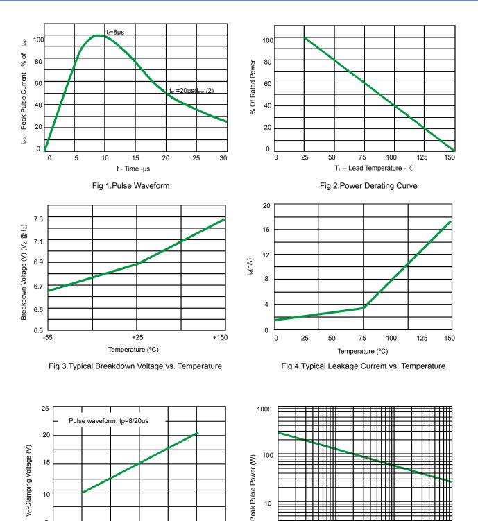
IPP-Peak pulse current (A) Fig 5. Clamping voltage vs. Peak pulse current
