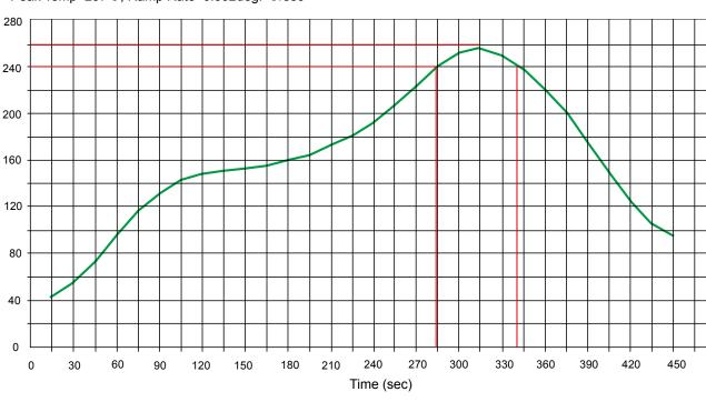
Peak Temp=257°C, Ramp Rate=0.802deg. °C/sec
