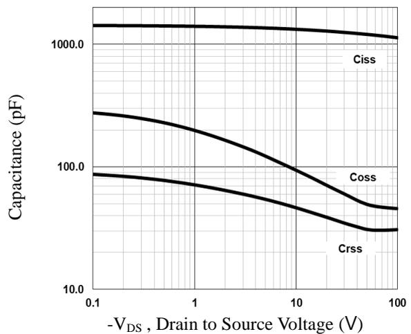
**Fig.6 Capacitance Characteristics**
