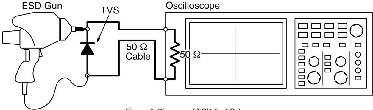
Figure 4. Diagram of ESD Test Setup
