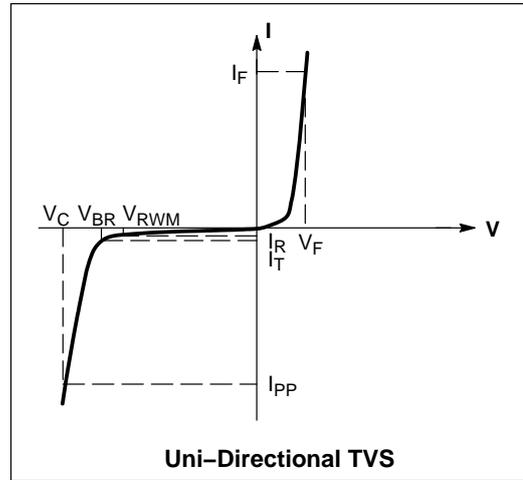
**ELECTRICAL CHARACTERISTICS** (T<sub>A</sub> = 25°C unless otherwise noted, V<sub>F</sub> = 1.1 V Max. @ I<sub>F</sub> = 10 mA for all types)
