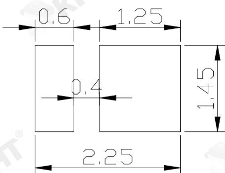
推荐焊盘式样(Recommended Soldering Patter)
