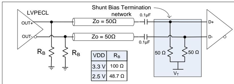
Figure 10. LVPECL and Low-swing LVPECL with AC-coupled Termination
