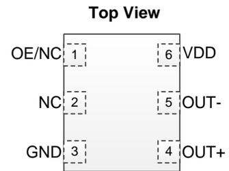
**Figure 3. Pin Assignments**
