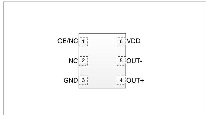
Figure 2. Pin Assignments (Top view)
