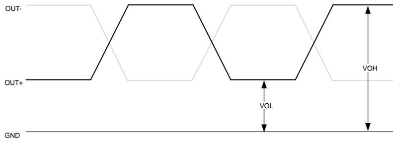
Figure 4. LVPECL, Low-swing LVPECL, and HCSL Voltage Levels per Differential Pin (i.e. OUT+, or OUT-)
