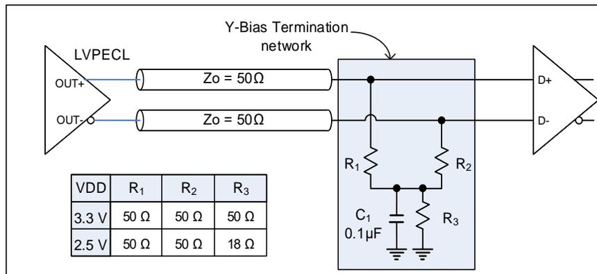
**Figure 12. LVPECL and Low-swing LVPECL with Y-Bias Termination**
