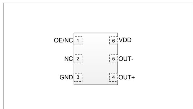
Figure 2. Pin Assignments (Top view)
