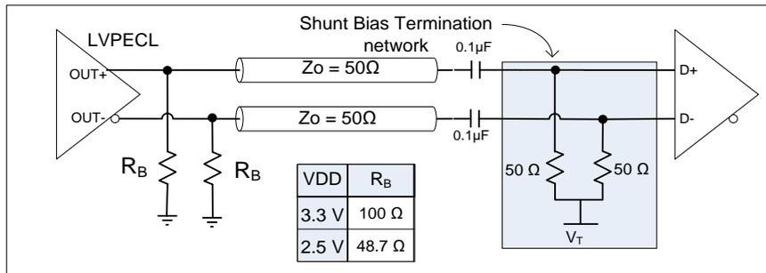
**Figure 10. LVPECL and Low-swing LVPECL with AC-coupled Termination**
