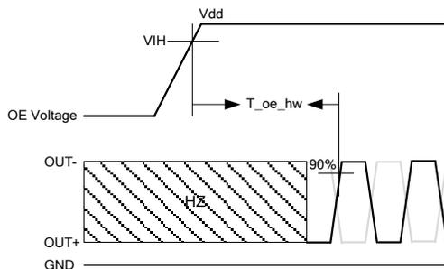
Figure 8. Hardware OE Enable Timing
