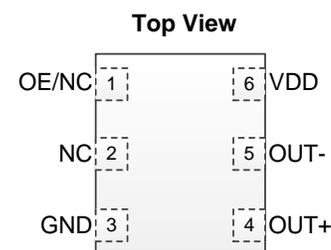
Figure 3. Pin Assignments
