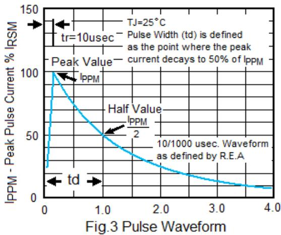
Fig. 3 Pulse Waveform
