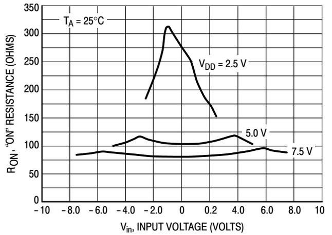
Figure 15. Comparison at  $25^\circ\text{C}$ ,  $V_{DD} = -V_{EE}$
