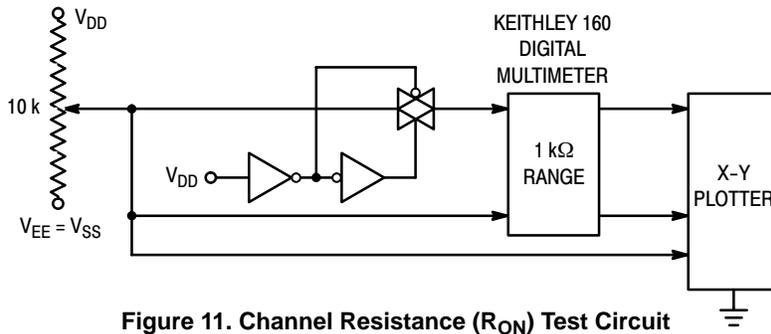
Figure 11. Channel Resistance ( $R_{ON}$ ) Test Circuit
