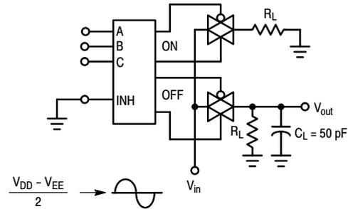
Figure 8. Channel Separation (Adjacent Channels Used For Setup)
