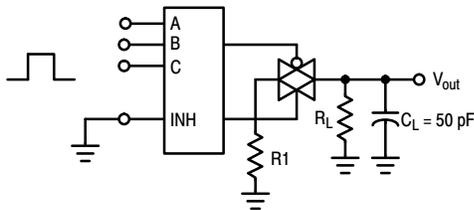
Figure 9. Crosstalk, Control Input to Common O/I
