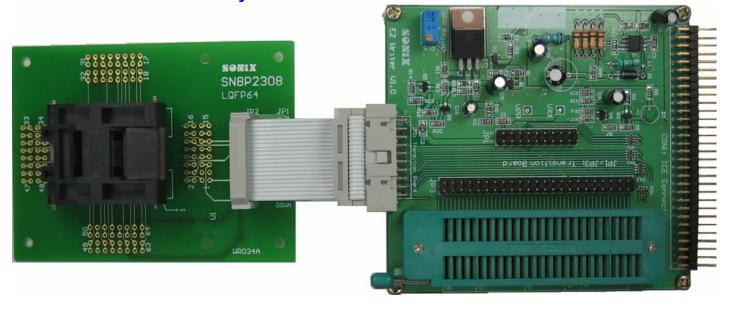
Note: Connect Easy Writer to ICE must be through an 60-pin cable
