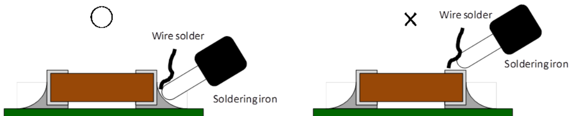
Fig 3 Correct handling method of soldering iron
