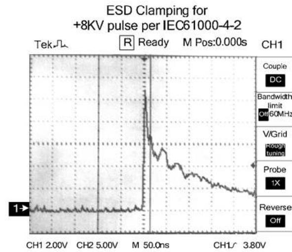
**LRC099-04DT1G****TYPICAL ELECTRICAL CHARACTERISTICS CURVE**
