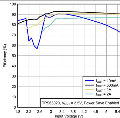
Figure 12. Efficiency Versus Input Voltage, TPS63020, V<sub>OUT</sub> = 2.5 V, Power Save Enabled
