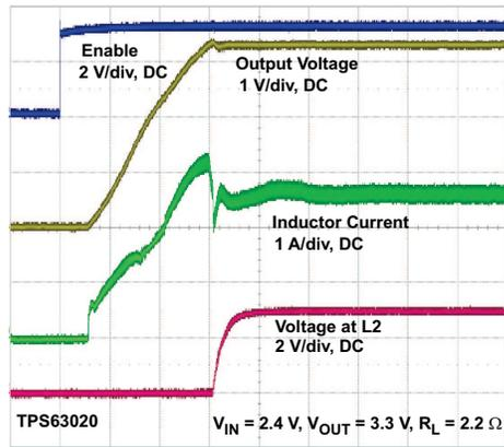
Figure 26. Start-up Behavior from Rising Enable, TPS63020
