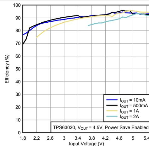
Figure 13. Efficiency Versus Input Voltage, TPS63020, V<sub>OUT</sub> = 4.5 V, Power Save Enabled
