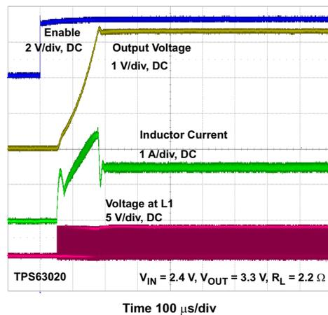
Figure 24. Start-up Behavior from Rising Enable, TPS63020
