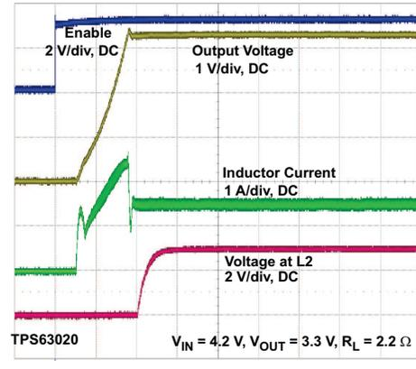
Figure 27. Start-up Behavior from Rising Enable, TPS63020
