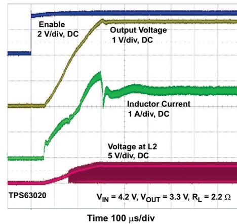
Figure 25. Start-up Behavior from Rising Enable, TPS63020
