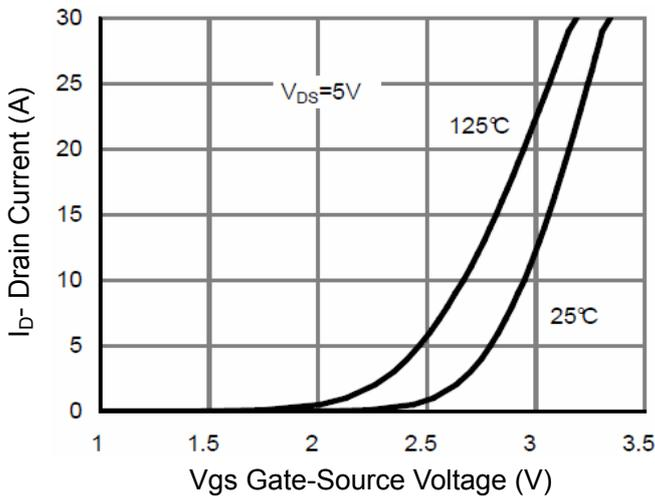
Figure 2 Transfer Characteristics
