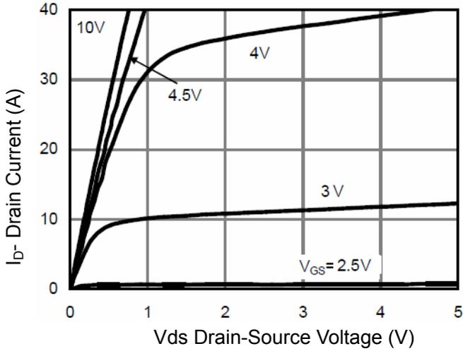
Figure 1 Output Characteristics
