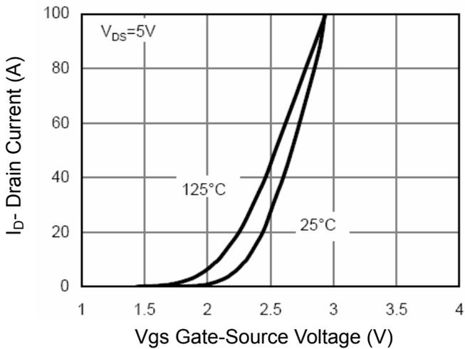
Figure 2 Transfer Characteristics
