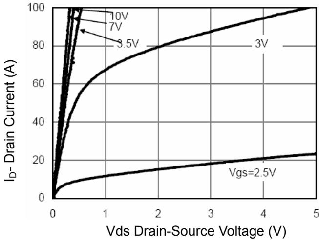
Figure 1 Output Characteristics
