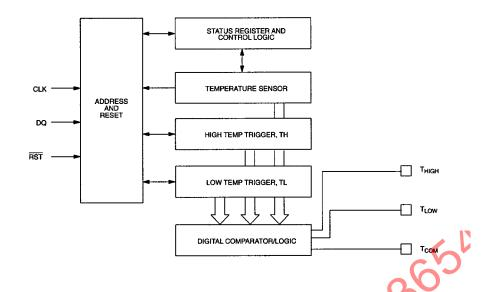
The DS1620 measures temperature using a bandgap-based temperature sensor. The temperature reading is provided in a 9-bit, two's complement reading by issuing a READ TEMPERATURE command. The data is transmitted serially through the 3-wire serial interface, LSB first. The DS1620 can measure temperature over the range of -55°C to +125°C in 0.5°C increments. For Fahrenheit usage, a lookup table or conversion factor must be used.
