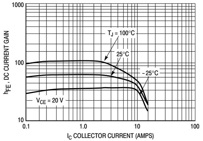
**Figure 4. DC Current Gain,  $V_{CE} = 20\text{ V}$**
