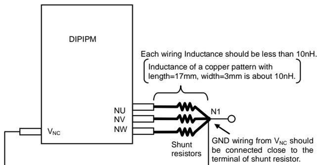
Low inductance shunt resistor like surface mounted (SMD) type is recommended.
