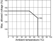
Note: The "Max. allowed voltage" is the maximum voltage that can be applied to the relay coil. It is not the maximum voltage that can be applied continuously.
